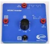
DC/AC inverters are used to convert the DC voltage of the solar module into an AC voltage to either feed the electricity into the grid or to operate customary domestic appliances in a smart-grid system. The leXsolar DC/AC inverter module does not produce mains voltage but an AC voltage with an amplitude of 2.5V and a variable frequency that can be adjusted with the potentiometer between 0.5
