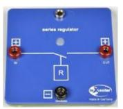
The leXsolar series regulator is a two-level regulator that disconnects the accumulator from the solar module when the charging voltage of 4.1V is reached. When discharging the accumulator the series regulator interconnects the input voltage of the solar module not before dropping below the lower threshold of 3.5V. The control LED is lighting as long as the series regulator is loading.
